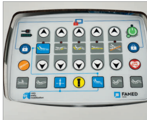
Central panel (supervisor) with VEM functions, one-button positions and electric CPR.
